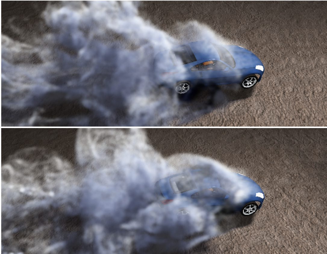
Figure 4.7: The wake behind a car is simulated with 1M particles. Our method (top) and the reference high-resolution solver (bottom) show similar small-scale details.
